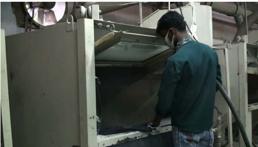
Sandblasting in Bangladesh using minimal Personal Protective Equipment. Credit: Altemeier & Hornung Filmproduktion
